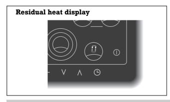
The residual heat display appears on the display of the relevant cooking zone after switching off.
